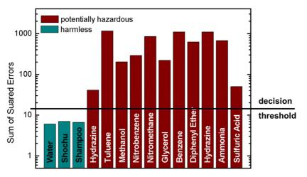
Figure 5: Definition of a decision threshold for a set of materials
