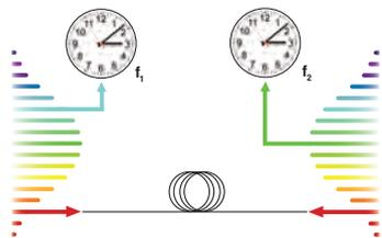
Lasers operating in the telecom range at 1550 nm and linked to stable optical clocks allow for the dissemination of ultrastable frequencies via optical fibers. Using optical frequency combs on both ends of the fiber connections and technologies for noise cancellation resulting from fiber length changes, stabilities better than  $10^{-16}$  in one second have been achieved in fiber networks over hundreds of kilometers.
